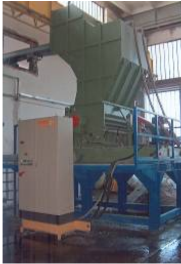
Picture 1: Wet shredder with knives, output 1-4 t/h
