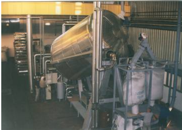
Picture 7: Vacuum crystallization equipment in operation
