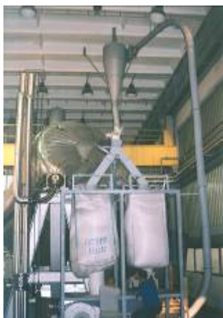
Picture 8: Vacuum crystallization equipment in production
